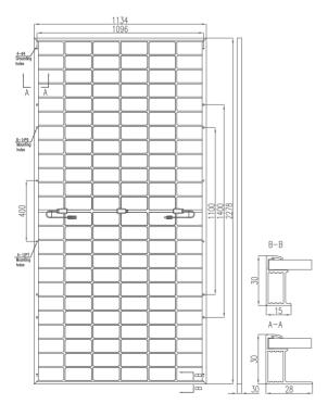
Note: 400mm hole distance is only applicable when specified by the customer
