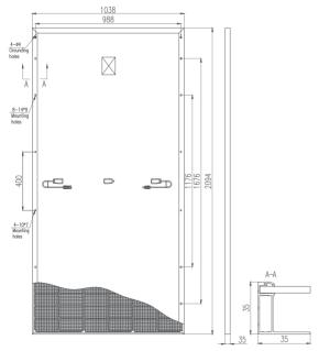
$^{*}$ 400mm mounting holes are only suitable for 6005-T6 aluminum frame
